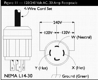
This receptacle powers 120/240 Volt AC, 60 Hz, single phase loads requiring up to 3,600 watts of power at 30 Amps for 120 Volts; 7,200 watts of power (7.2 kW) at 30 Amps for 240 Volts. The outlet is protected by a 30 Amp push-to-reset circuit breaker.
